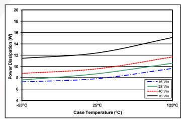
*Figure 6*: Power dissipation at 60% load (2.4A load on +15V and 2.4A load on -15V) versus case temperature for Vin =16V, 28V, 40V, and 70V.
