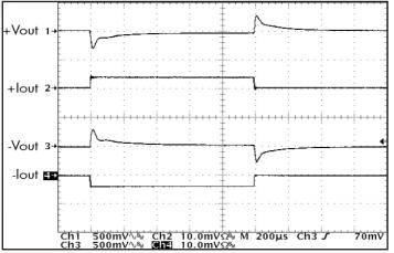
**Figure 18**: Output voltage response to step-change in total load current (0%-50%-0%) of total lout (max) split 50%/50%. Load cap:  $1\mu F$  ceramic cap and  $10\mu F$ ,  $100m\Omega$  ESR tantalum cap. Ch 1: +Vout (500mV/div); Ch 2: +Iout (5A/ div); Ch 3: -Vout (500mV/div); Ch 4: -Iout (5A/div).
