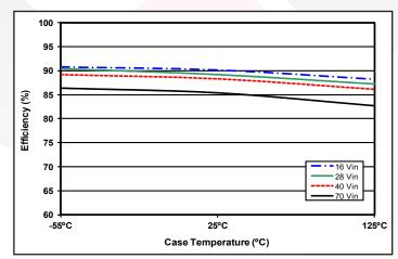
*Figure 5*: *Efficiency at 60% load (2.4A load on +15V and 2.4A load on -15V) versus case temperature for Vin = 16V, 28V, 40V, and 70V.*
