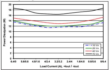
*Figure 4*: Power dissipation vs. output current, with total output current fixed at 80% load (96 W) and loads split as shown between the +15V and -15V outputs at minimum, nominal, and max input voltage at 25°C.
