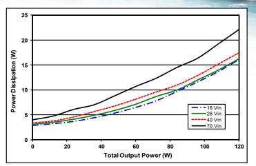
Figure 2: Power dissipation vs. output power, from zero load to full load with equal load on the +15V and -15V outputs at minimum, nominal, and maximum input voltage at  $25^{\circ}$ C.
