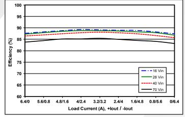
**Figure 3**: Efficiency vs. output current, with total output current fixed at 80% load (96 W) and loads split as shown between the +15V and -15V outputs at minimum, nominal, and maximum input voltage at 25°C.
