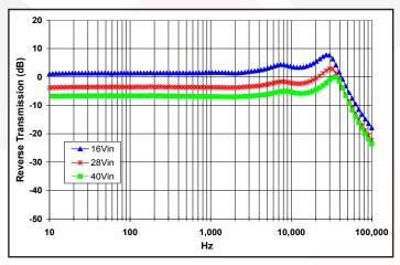
**Figure 29**: Magnitude of incremental reverse transmission from +15V output (+RT = iin /+iout) for minimum, nominal, and maximum input voltage at full rated power.
