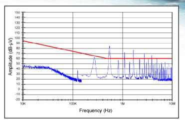
*Figure 32*: High frequency conducted emissions of standalone MQFL-28-05S, 5Vout module at 120W output, as measured with Method CE102. Limit line shown is the 'Basic Curve' for all applications with a 28V source.
