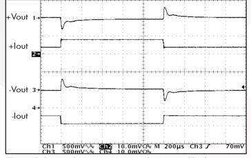
**Figure 17**: Output voltage response to step-change in total load current (50%-100%-50%) of total lout (max) split 50%/50%. Load cap:  $1\mu$ F ceramic cap and  $10\mu$ F,  $100m\Omega$  ESR tantalum cap. Ch 1: +Vout (500mV/div); Ch 2: +Iout (5A/div); Ch 3: -Vout (500mV/div); Ch 4: -Iout (5A/div).
