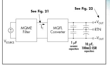
*Figure 20*: Test set-up diagram showing measurement points for Input Terminal Ripple Current (Figure 21) and Output Voltage Ripple (Figure 22).
