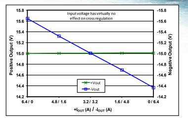
**Figure 8**: Load regulation vs. load current with power fixed at 80% load (96W) and load currents split as shown between the +15V and -15V outputs, at nominal input voltage and Tcase =  $25^{\circ}$ C.
