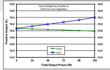
**Figure 9**: Load regulation vs. total output power from zero to to full load where +lout equals three times -lout at nominal input voltage and Tcase =  $25^{\circ}$ C.
